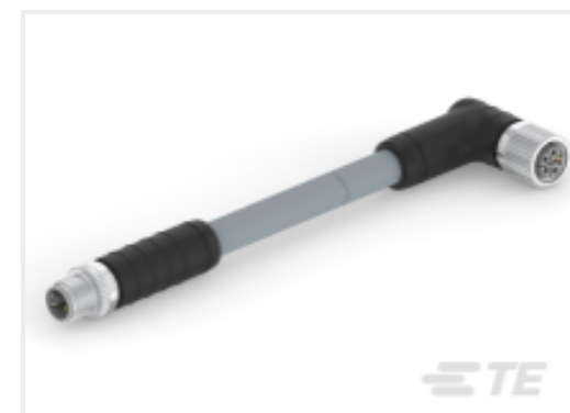
TE Part # CAT-SI113-M1ZZO M12 L-code 5pin male straight to female right angle, PVC gray 14 AWG
