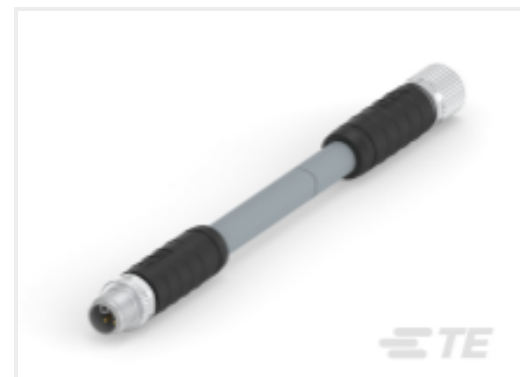
TE Part # CAT-SI113-M1ZP M12 L-code 5pin male straight to female straight, shielded polyurethane gray 14 AWG
