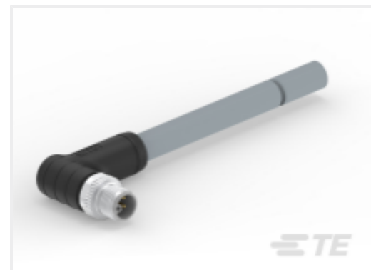
TE Part # CAT-SI113-M1ZD M12 L-code 5pin male right angle pigtail, shielded polyurethane gray 14 AWG
