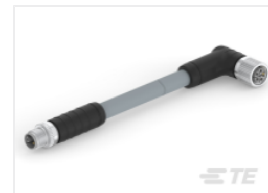
TE Part # CAT-SI113-M1ZN M12 L-code 5pin male straight to female right angle, polyurethane gray 16 AWG
