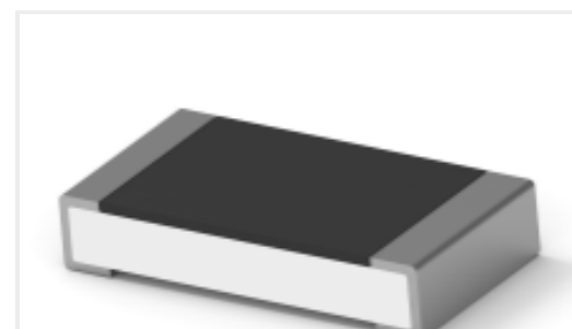
TE Part #4-2176391-7 RQ 1206 37K4 0.1% 10PPM 5K RL
