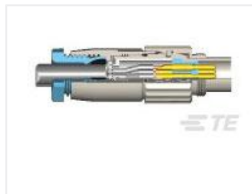
TE Part #1-1437719-1 T01-0540-P03-MALE PLUG CONNECTOR-CRIMP
