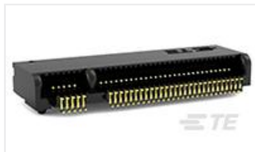
TE Part #2199119-4 M.2 0.5PITCH 3.2H KEY E 15U" AU
