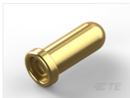
TE Part # CAT-377-MSSCB75 Miniature Spring Sockets: Closed Bottom, Beryllium Copper, 7.5A
