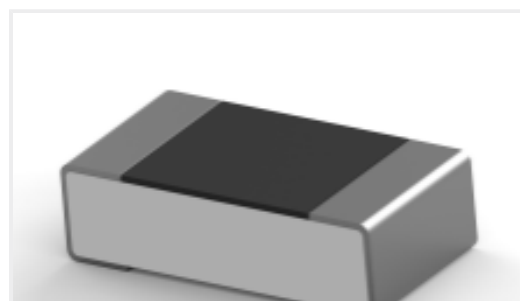
TE Part #7-2176367-4 RQ 0603 26K7 0.1% 10PPM 1K RL
