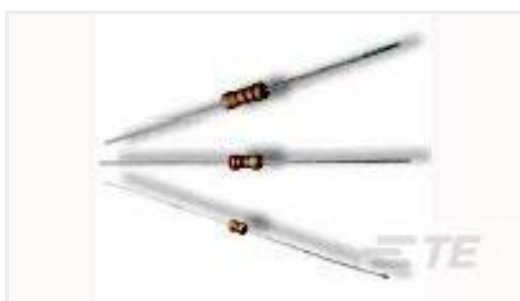
TE Part #1623931-9 CFR25 5% 33R
