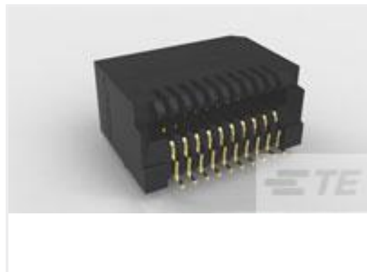
TE Part #1888247-1 20 POS SMT CONN, SFP/SFP+, 30A
