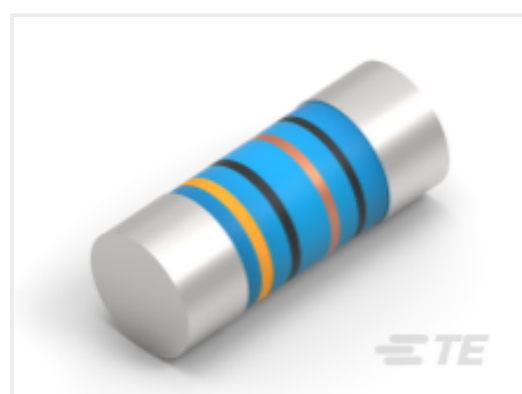
TE Part #4-2176315-5 MELF SMA_A 390R 1% 50PPM 0204 0.4 W
