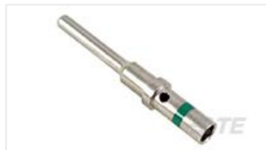
TE Part #0460-215-16141 PIN, SOLID, SIZE 16, 14AWG, NI
