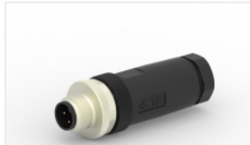
TE Part #T4111002041-000 M12,MALE,STRAIGHT,A CODE,4P, PG9,GOLD
