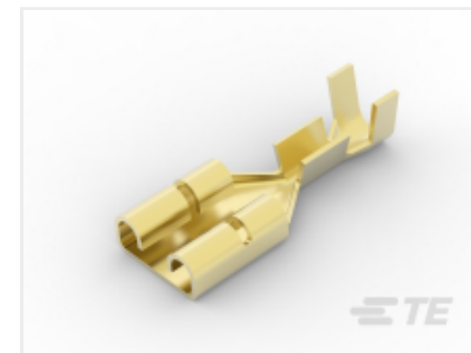
TE Part # 63609-1 250 FASTON REC 22-18 AWG BR
