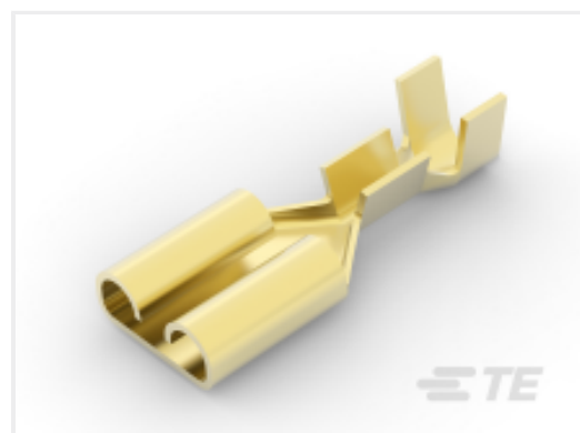
TE Part # 2238027-3 250 FASTON,REC.,22-18 AWG,BR
