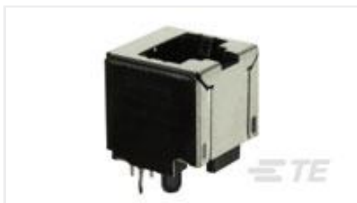
TE Part #6368150-1 MJ, TE, 8P, CAT5, SHIELDED
