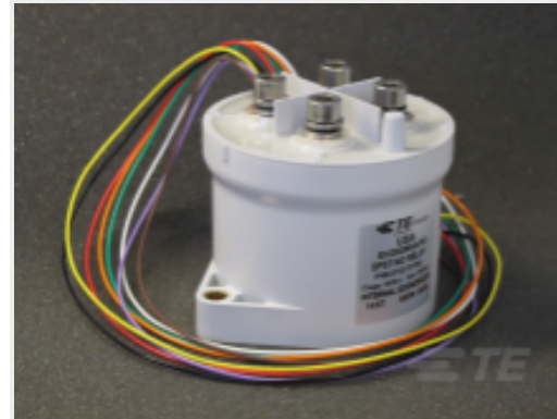
TE Part # 9-1618406-9 EV202AVAND=RELAY, DPST-NO 12Vdc
