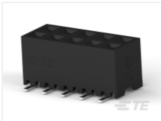
TE Part # 1-2314845-0 10P,2MM,BB,REC,DRVT,SMD,AU.38, TB,W/CP
