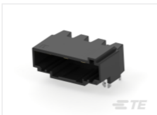
TE Part #CAT-D9934-A75I Header Assembly: Wire-to-Board Connector, Spring Clamp, 7.5 mm pitch, 14.5A
