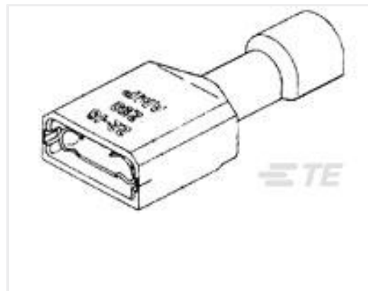
TE Part #2-520184-2 ULTRAFAST 250 ASSY REC 22-18 TPBR LP
