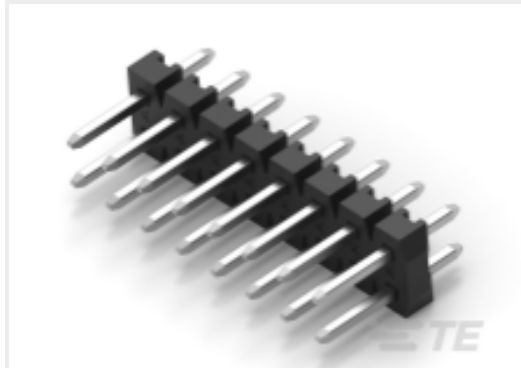
TE Part # 2842139-7 14P,2MM,BRK HDR,DRVT,2.8,0.38AU, BOX
