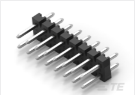
TE Part # 2842127-7 14P,2MM,BRK HDR,DRVT,2.8,0.38AU, TB
