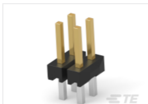
TE Part #2823124-4 4P,2MM,BRK HDR,DRVT,2,8,0.76AU,TB
