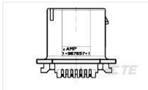
TE Part #1-967657-1 4pos MQS 0.63 header 90deg
