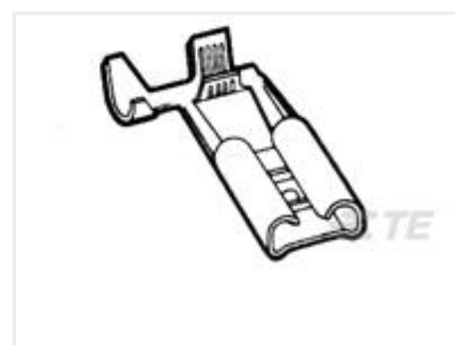
TE Part #1-280050-2 250 FASTON, FLAG, REC., 16-20 AWG, TPBR
