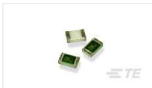
TE Part #2-1879223-7 CPF 0603 442R 0.1% 25PPM 1K RL
