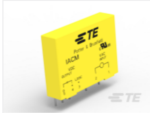
TE Part # 9-1393028-0 IACM-24E =SLIM PCB MONT,24VDC Logi-AC ip
