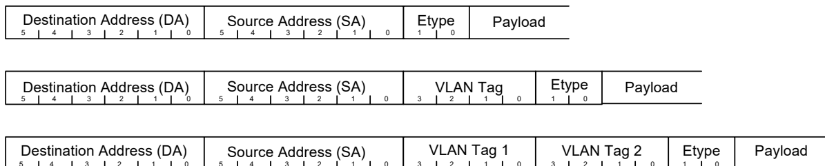
Figure 44 • Type II Ethernet Basic Frame Format
