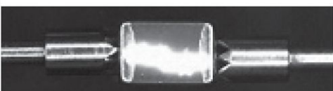
Standard Capacitor with Surface Arc-over
