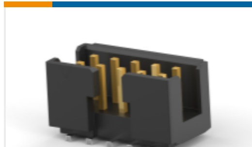
TE Part #1-2373376-0 10P,2MM,SHRD HDR,DRV,T,SMD,0.1 AU,TB
