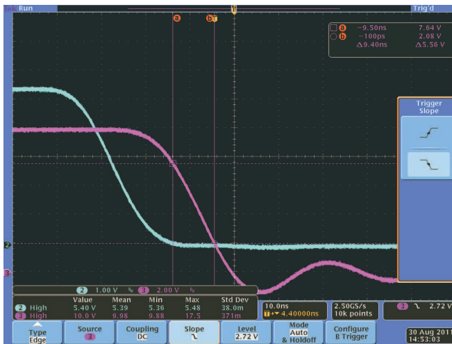
Figure 25. Typical Turn-On Waveform (VDD = 10 V, C L = 1 nF)
