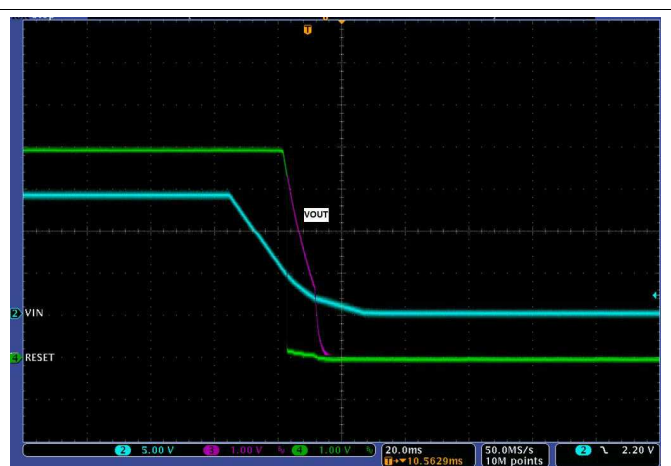
Figure 24. TPS7B6750-Q1 Power-Down Waveform
