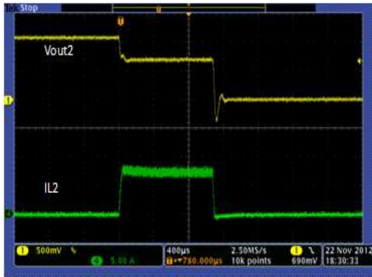
Figure 29. Over Current Protection, Buck2
