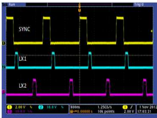
Figure 31. Synchronization at 500 kHz
