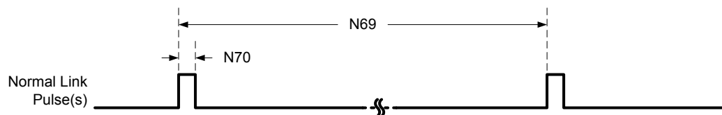
Figure 31-38. 10Base-TX Normal Link Pulse Timing
