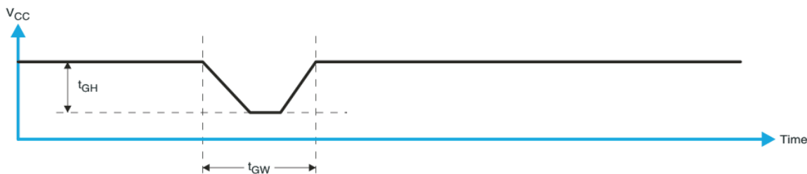
Figure 14. Glitch Width and Glitch Height
