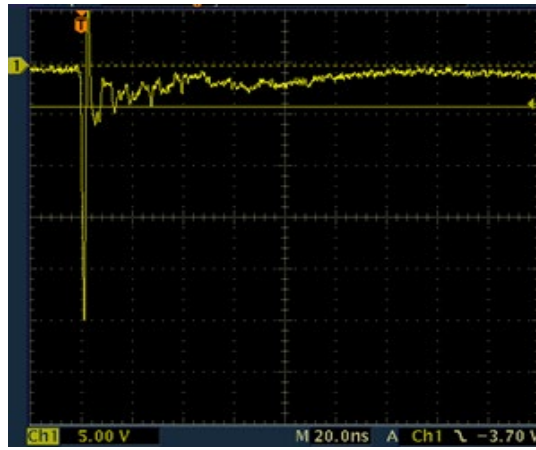
SP1105S IEC 61000 -4-2 -8 kV Contact ESD Clamping Voltage
