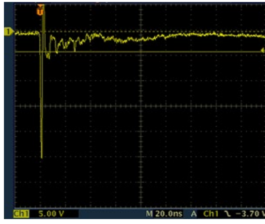
SP1112 IEC 61000 -4-2 -8 kV Contact ESD Clamping Voltage
