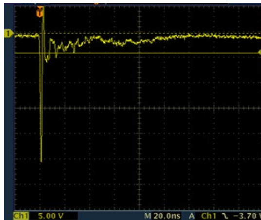
SP1112 IEC 61000 -4-2 -8 kV Contact ESD Clamping Voltage
