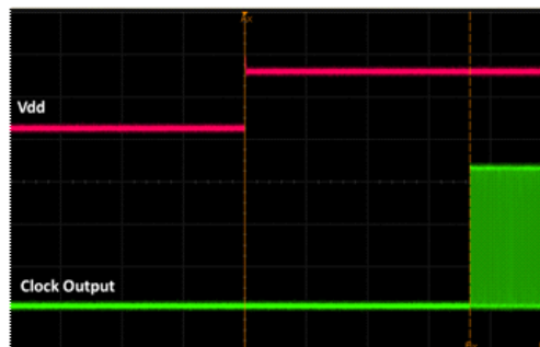
Figure 16. Startup Waveform vs. Vdd
