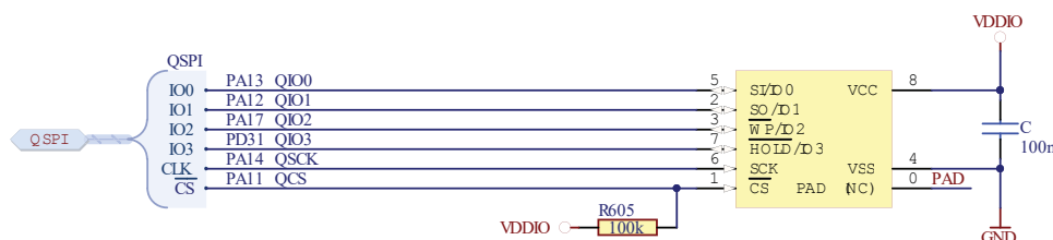
Figure 58-6. Schematic Example with QSPI Data Flash
