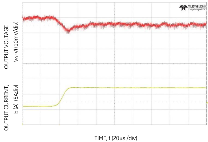
Figure 4. Transient Response to Dynamic Load Change from 50% to 100% at 12V in , C out =4x47uF+6x330uF, C Tune =47nF, R Tune =300
