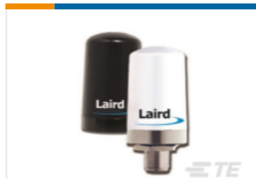
TE Part #TRAB24-49003P OMNI,Ph,2400/4900MHz BK,3 dBi, 60W,
