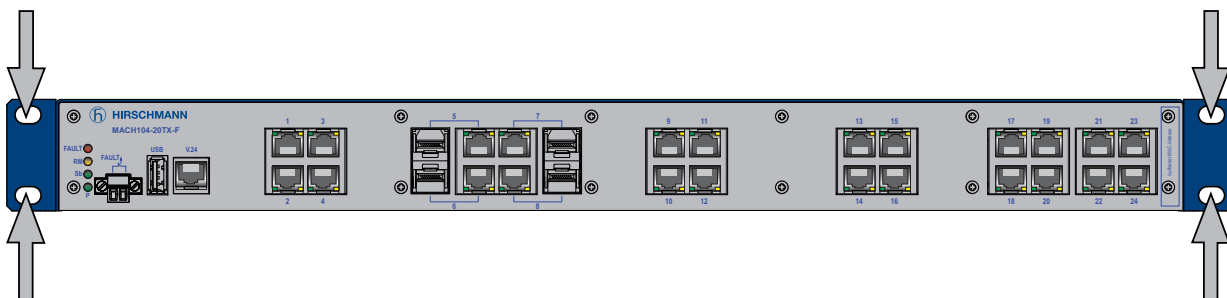
Figure 13: Mounting the MACH104 in the 19" cabinet
