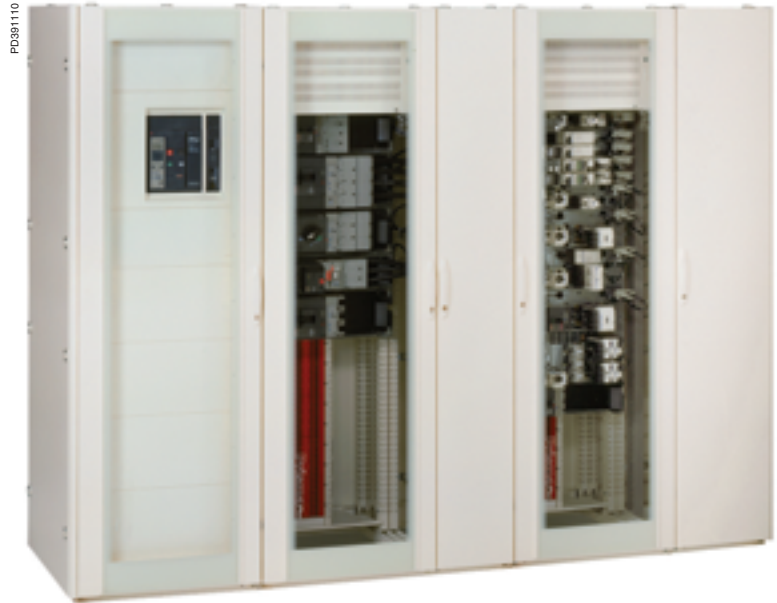
All cover panels and doors IP30 are secured using quarter-turn fasteners. Electrical continuity is achieved naturally, without having to add clips or earthing braids.
