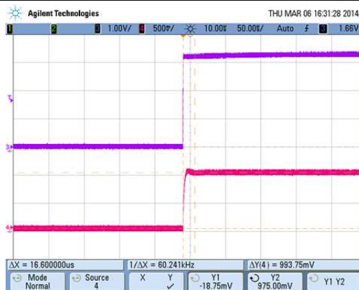
VDD=3.3V Top trace is T_ON Bottom trace is TAO
