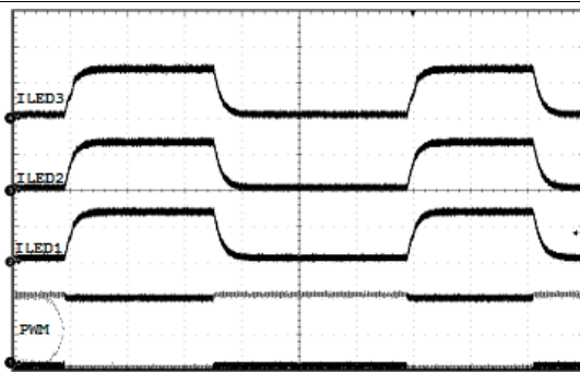
Figure 52. Led Current Ripple vs F_{PWM}
