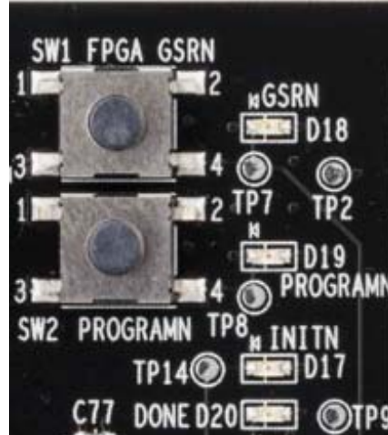
Figure 3. ECP5 Status LEDs and Push-button Controls
