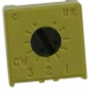
363 Series Trimmer, 20 kOhm, 0.5 W, 1 Turns, Square Body, Vertical Shaft
