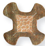
Indenter Crimp Cross-Section Across Axis Figure 2
