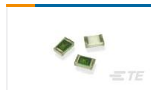
TE Part #1-2176092-8 RP 2A 0.25W 1K0 0.1% 25PPM 1K RL
