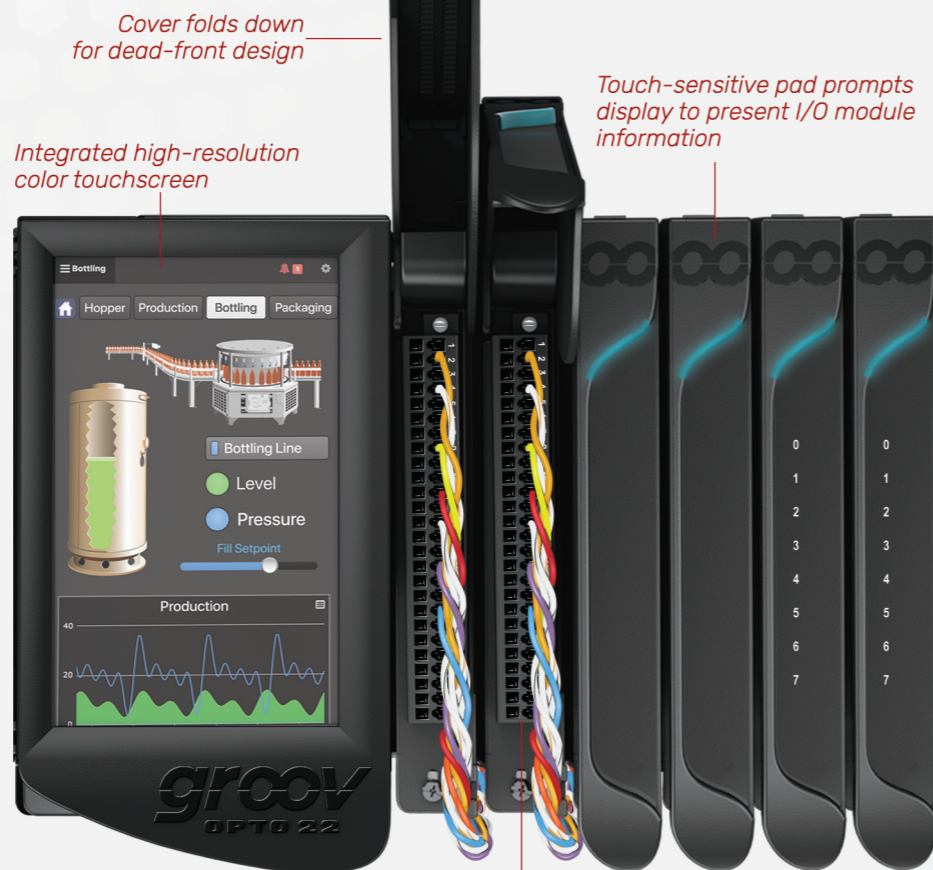
Integrated wireway with hinged 2-position cover
