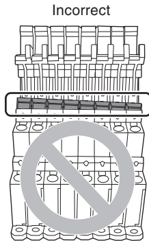
Incorrect installation Some terminals not inserted completely. Incorrect
