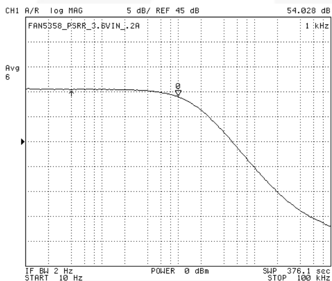
Figure 19. Power Supply Rejection Ratio at 200mA Load
