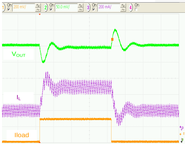
Figure 15. Load Transient 200 to 500mA, 3.6VIN, 5µs/div.
