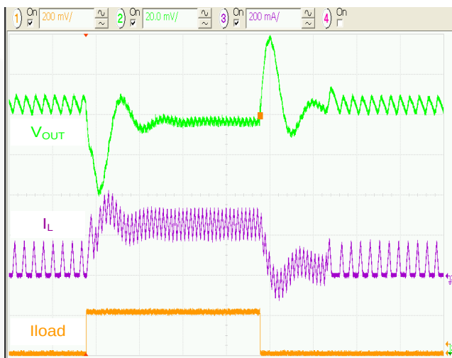
Figure 14. Load Transient 50 to 250mA, 3.6VIN, 5µs/div.
