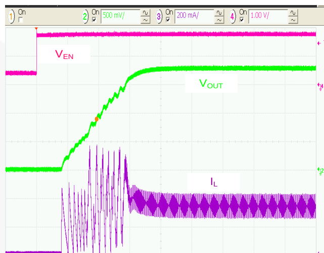
Figure 18. Soft-Start, R_{LOAD} = 6\Omega , 20µs/div.
