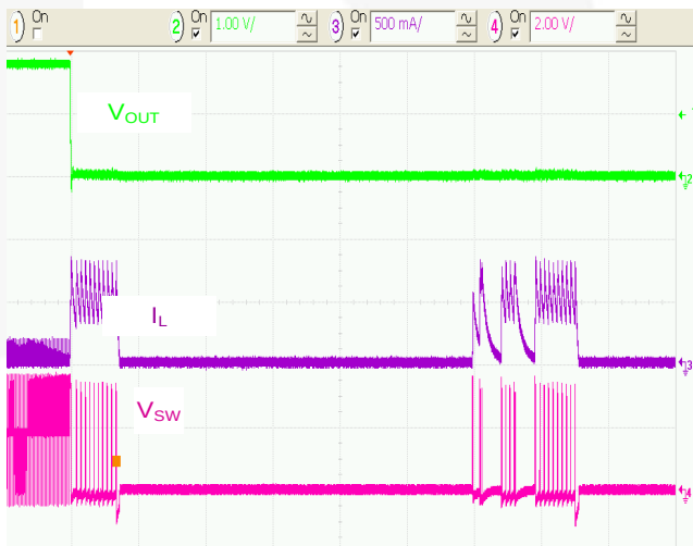
Figure 16. Metallic Short Applied at VOUT, 50µs/div.
