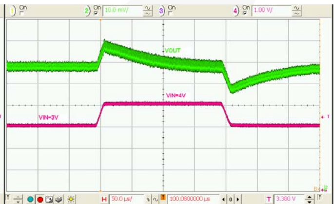
Figure 21. Line Transient, I_{LOAD}=1.0\text{ A} , t_R=t_F=10\ \mu\text{s}
