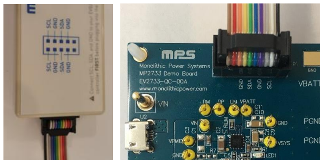
Figure 6: EVB to MPS I 2 C Communication Interface Wire Connection
