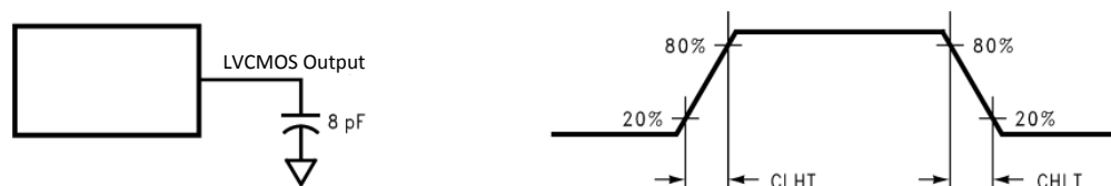
Figure 2. LVC MOS Output Load and Transition Times
